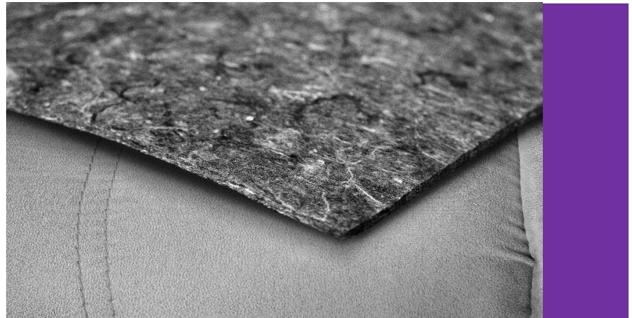
**Characteristic:** Nonwoven textile mechanically bonded by needle punching and coated
